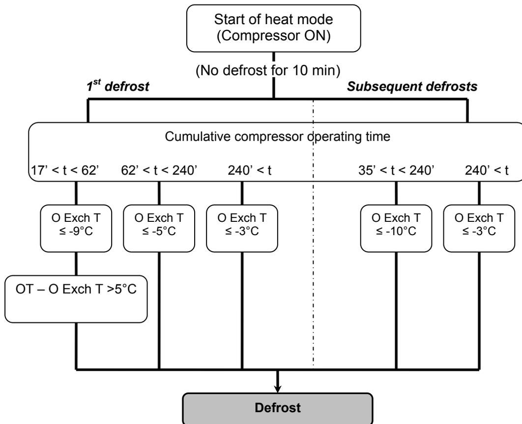
O Exch T : outdoor unit exchanger temperature
