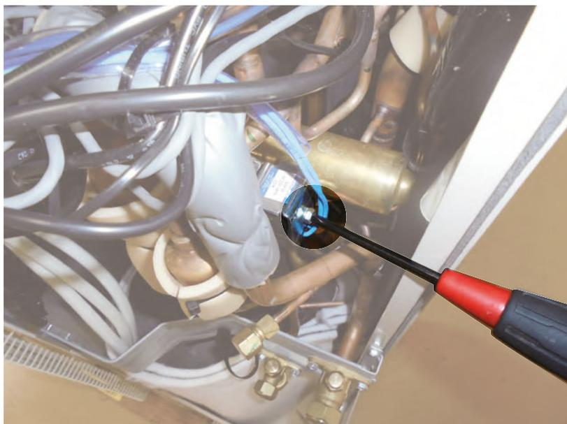
Remove the mounting screw with wrench or short screwdriver.
