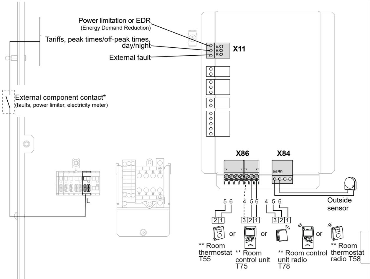
\* If the control device does not provide a potential-free contact, the contact must be relayed to create equivalent wiring. In all cases, please refer to the instruction manuals for the external components (load shedder, power meters) to create the wiring.
