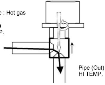
There is no refrigerant flow coming to EEV(INJ) while the liquid injection is inactive. Check whether the liquid injection is active before executing check point 5 for EEV(INJ).
