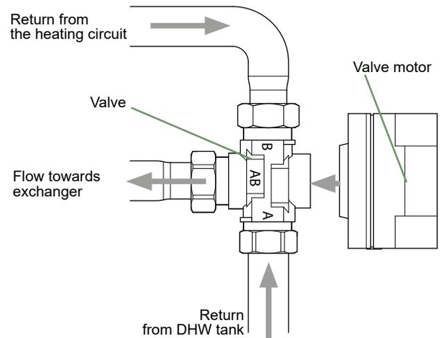
fig. 6 - Mounting the distribution valve
