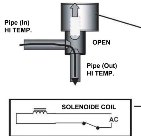
☒ If the valve closes by removing the connector of the valve which does not close, it is considered to be Main PCB failure. Replace Main PCB.
