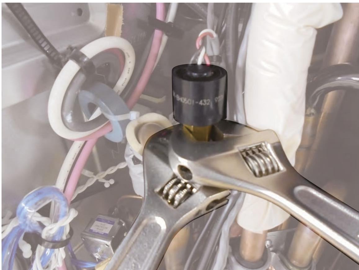
**Remove the PRESSURE SENSOR with wrench.**
