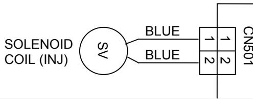
**Check point 2 : Check solenoid coil**
