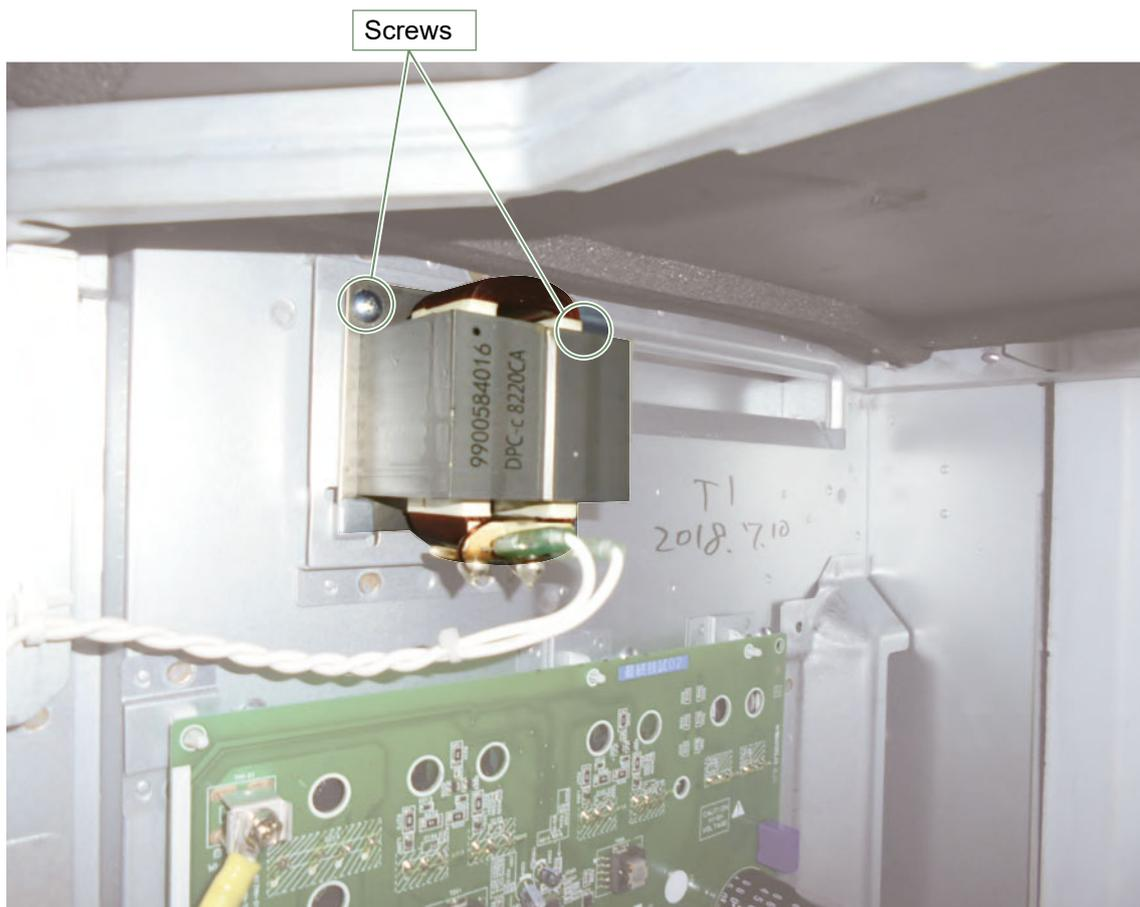
Remove the wire and mounting screw.
