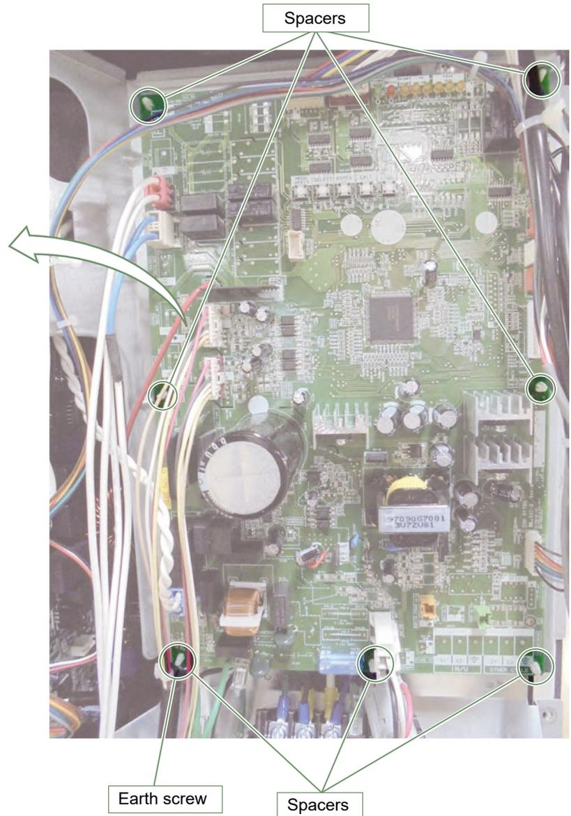
Remove the communication cable connected to the terminal.
