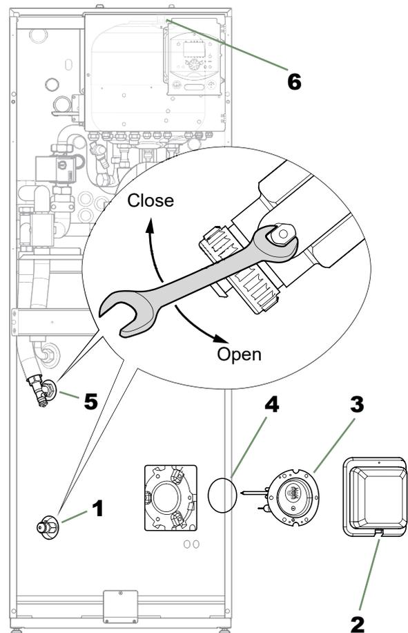
fig. 5 - Draining the hydraulic unit and/or hot water tank
