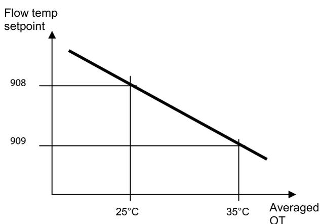
The cooling characteristic is adjusted for a 25 °C room temperature setpoint. If the room temperature setpoint is changed the curve will automatically adapt.
