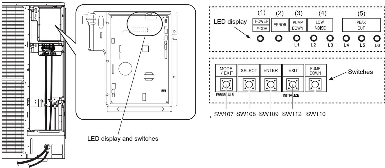
fig. 8 - Location of switches and LED on outdoor unit
