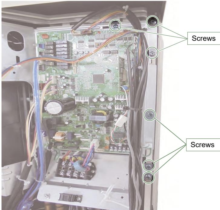
Remove the 6 mounting screws.
