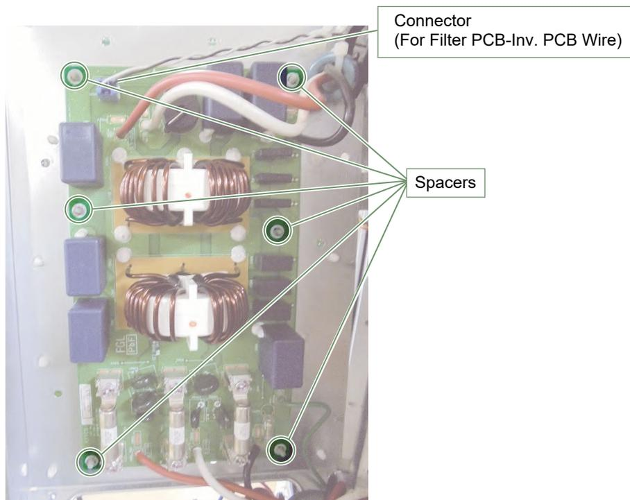
Remove the connector (Filter PCB - Inverter PCB wire).
