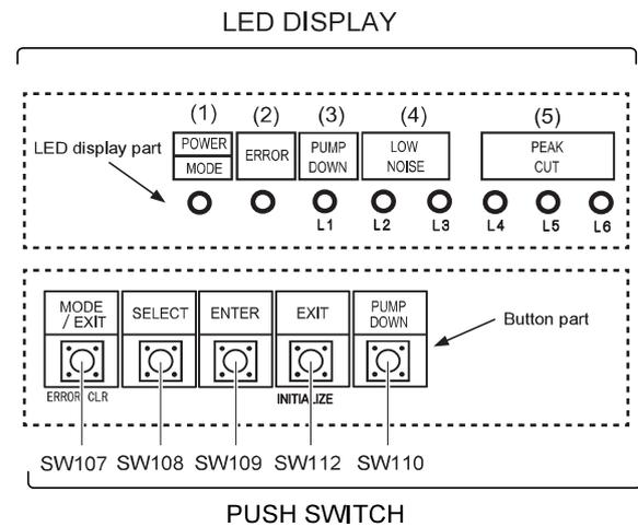
*fig. 3 - Location of switches and LED on single phase and 3-phases outdoor unit*
