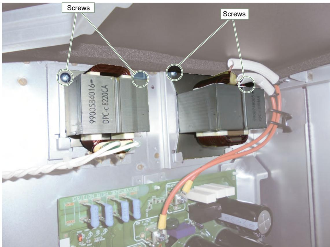
Remove the wire and mounting screw.
