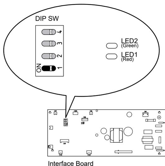
fig. 1 - Location of DIP switches and diodes on the hydraulic unit interface card
