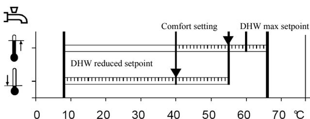
The DHW is heated to various setpoint values. These setpoints are active according to the selected operating mode and allow the desired temperatures to be reached in the DHW storage tank.
