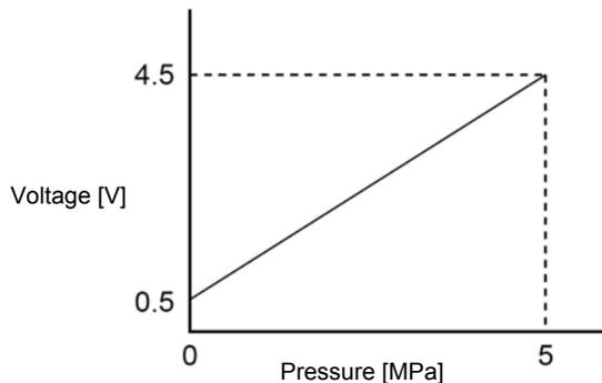
If the voltage is not correct, replace Presure Sensor.
