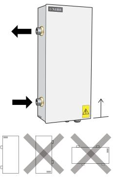
The immersion heater must be installed standing (see image above). An area of 500 mm is required in front of the immersion heater for service work. If this is not possible, detachable connections should be used.
