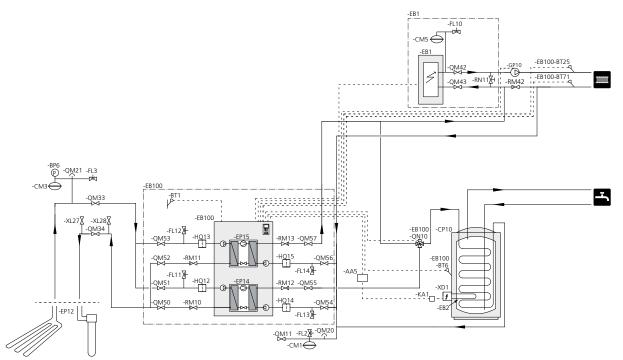
Module EP14 prioritises hot water charging via a reversing valve. When the hot water heater/accumulator tank is fully charged, the reversing valve switches to the heating circuit. The heat pump is controlled by an outdoor sensor combined with the flow line sensor which must be placed on the main pipe to the radiators. ELK 26 is connected automatically when the energy requirement exceeds the heat pump capacity.
