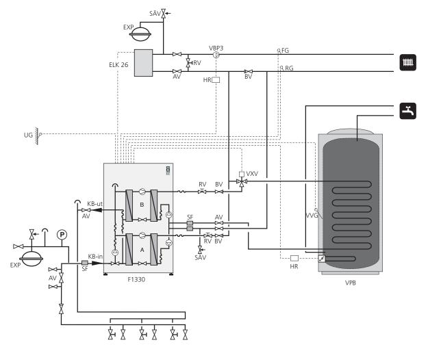
FIGHTER 1320/1330 / F1330 prioritises loading of hot water with half the output (heat pump module B) via a reversing valve. When the hot water heater/accumulator tank is fully charged, the reversing valve switches to the heating circuit.
